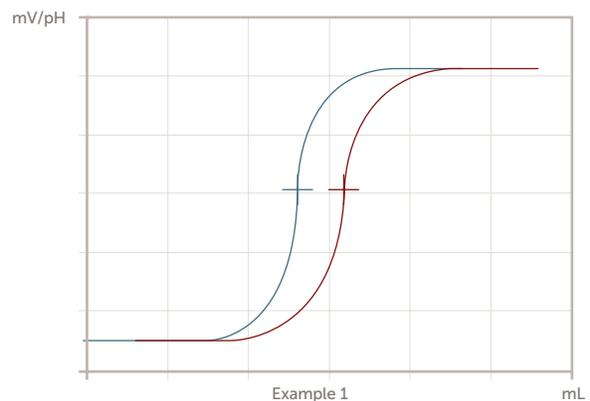
Example 1 shows a curve shifted to the left (in blue). This would be shown as a lower than expected result. The possible causes are, 1. the process itself has a lower concentration and the SemiChem APM 200 reports the correct result, 2. possible air bubble in the sample causing a lower than expected value, 3. a stronger titrant it being used resulting in less being required to reach the end point. Note the initial mV and titration end are the same. This indicates the chemistry is working.
