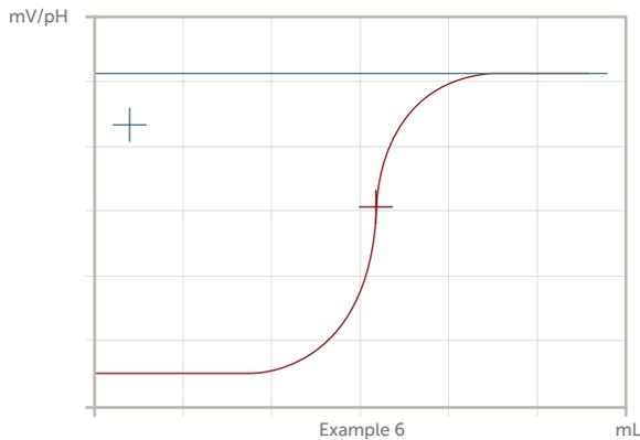
Example 6 shows a sensor response above the programmed end point. The user would not see this because the SemiChem APM 200 will abort the analysis and report an error code 1 or 2. A possible cause is the cell did not drain and flush properly.
