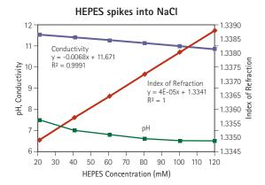
Figure 1: pH, conductivity and Entegris IoR outputs are shown versus HEPES concentration in mM. Six HEPES concentration spikes of 20 mM were added into the sodium chloride solution for a total HEPES concentration of 120 mM in NaCl.
