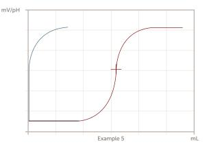
Example 5 shows an immediate change in sensor response. The possible causes are, 1. no sample, 2. very strong reagent, 3. very weak sample.
