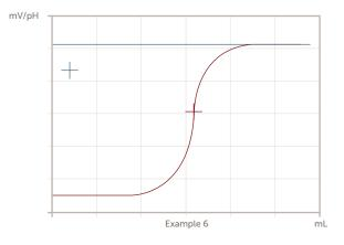
Example 6 shows a sensor response above the programmed end point. The user would not see this because the SemiChem APM*i* 200 will abort the analysis and report an error code 1 or 2. A possible cause is the cell did not drain and flush properly.
