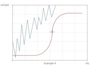
Example 4 shows a noisy signal from the sensor. Possible causes are, 1. malfunctioning electronics, 2. disconnected sensor, 3. incorrect sensor, 4. electrode not immersed in the sample, 5. low electrolyte in the sensor.
