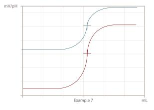
Example 7 shows a sensor response that is above the expected mV range. Possible causes are, 1. incorrect set-up parameters, 2. incorrect sensor calibration, 3. electrode drift outside of the end point window.
