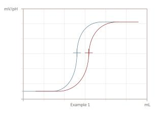
Example 1 shows a curve shifted to the left (in blue). This would be shown as a lower than expected result. The possible causes are, 1. the process itself has a lower concentration and the SemiChem APM*i* 200 reports the correct result, 2. possible air bubble in the sample causing a lower than expected value, 3. a stronger titrant it being used resulting in less being required to reach the end point. Note the initial mV and titration end are the same. This indicates the chemistry is working.
