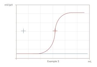
Example 3 shows a flat line indicating no response from sensor. The possible causes are, 1. no reagent, 2. a very weak reagent, 3. the wrong reagent, 4. a very strong sample, 5. malfunctioning reagent dispenser. This scenario would most likely be accompanied with an error code 8. Since the initial millivolts are consistent, most likely the sensor and associated electronics are performing properly.
