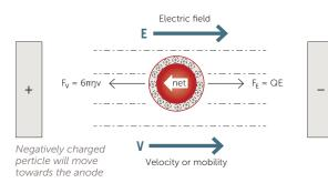
*Figure 5. Electrophoretic Light Scattering (ELS) technique. Source: Entegris*  The direction indicates if the particles are positively or negatively charged. The speed of the particles indicates the magnitude of the charge. Particle velocity can be measured using either phase analysis light scattering (PALS) or using frequency analysis. PALS is the newer, more sensitive approach and is now the preferred method for most samples.
