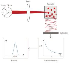
Figure 4. Optical diagram of a DLS system. Source: Entegris
