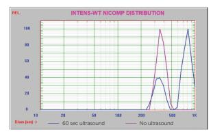
Figure 6. No ultrasound vs. 60 sec ultrasound
