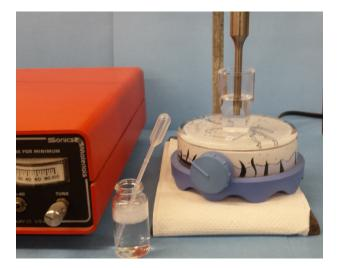
A well organized particle size laboratory should include some of the basic supplies mentioned in this document, such as a range of chemicals, solvents, surfactants, and an ultrasonic probe when dispersing powder.
