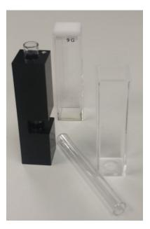
Figure 7. Clockwise starting at the top; 10 mm glass cell, 10 mm disposable plastic cell, round glass cell, round glass cell inside metal cell holder
