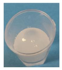
Figure 1. Poor sample powder wetting
