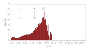
Figure 9. GMV liposome after extrusion through 5 μm filter.
