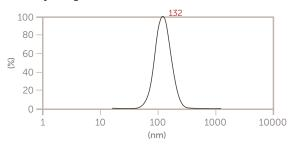
Figure 6. Liposome size after extrusion through 0.1  $\mu$ m membrane three times.
