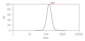
Figure 5. Liposome size after extrusion through 0.4  $\mu m$  membrane three times.
